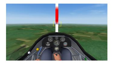
2. After passing the red/white pole, direct the glider's flight path to the center of the window by holding the yaw string horizontally within the sides of the window, and holding the 42-knot IVR (top edge of the yaw string tape) on the vertical center of the window.
