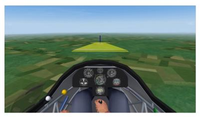
The glide slope appears to intersect the ground at the point of zero-parallax. During a descent, this point appears to remain stationary in the pilot's field of view.
