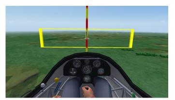
9. Establish and stabilize a 56-knot descent toward the window with the dive brakes closed.
