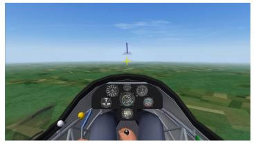
At the left, the glider is flying at the 38-knot angle of attack with the dive brakes partially deployed. Sighting through the IVR helps the pilot visualize the glide path.
