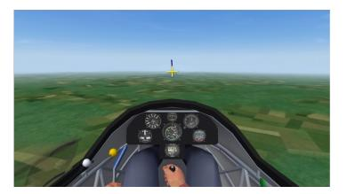
In the image to the left, the pilot has altered the descent profile by opening the dive brakes.
