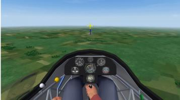
In a descent, the same IVR represents the flight path at the 56-knot angle of attack.
