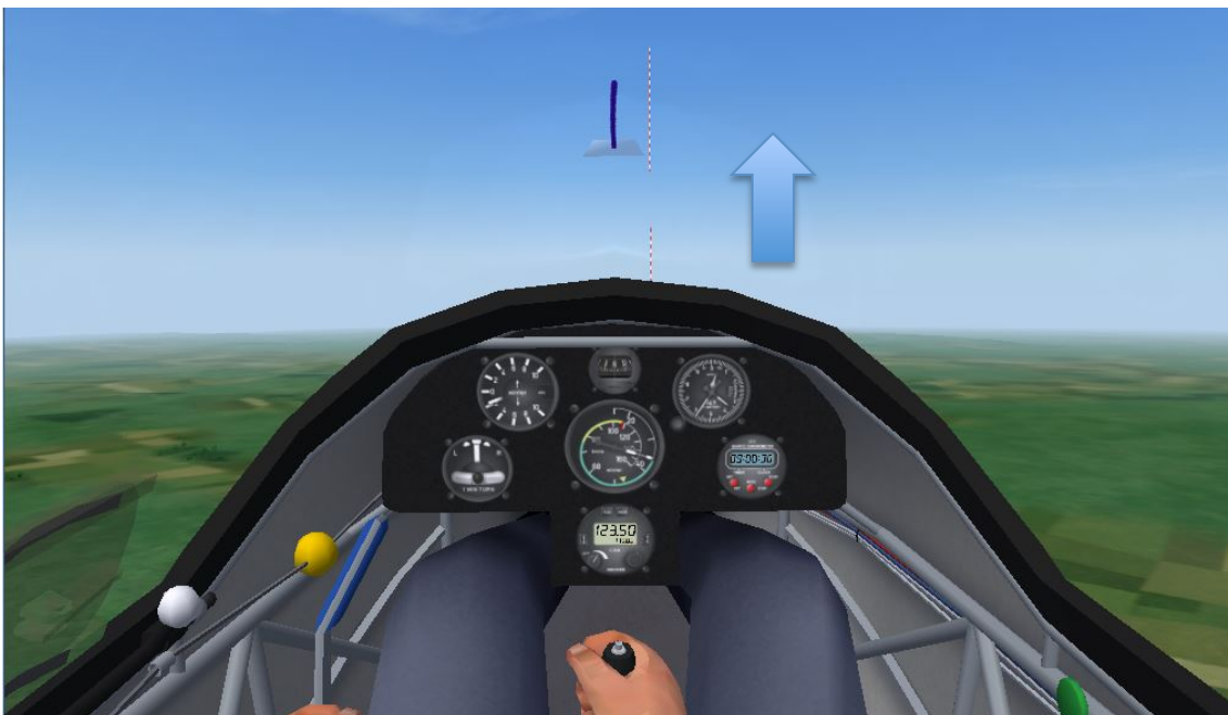
Initial pitch above the attitude required for 32 knots
