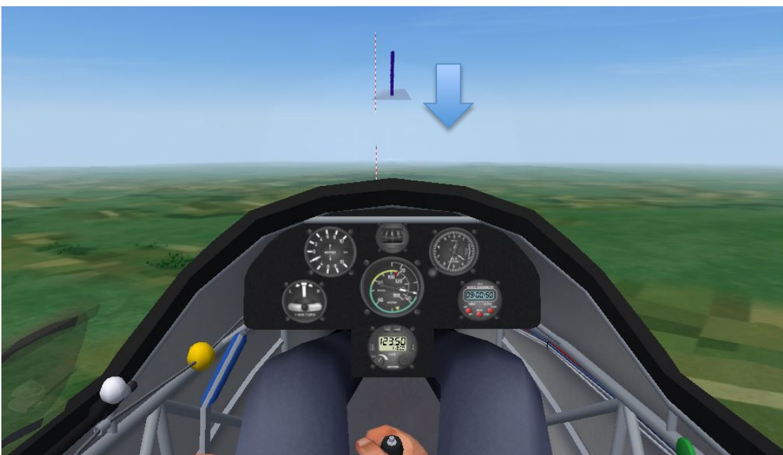
Secondary pitch to capture/hold the attitude for 32 knots
