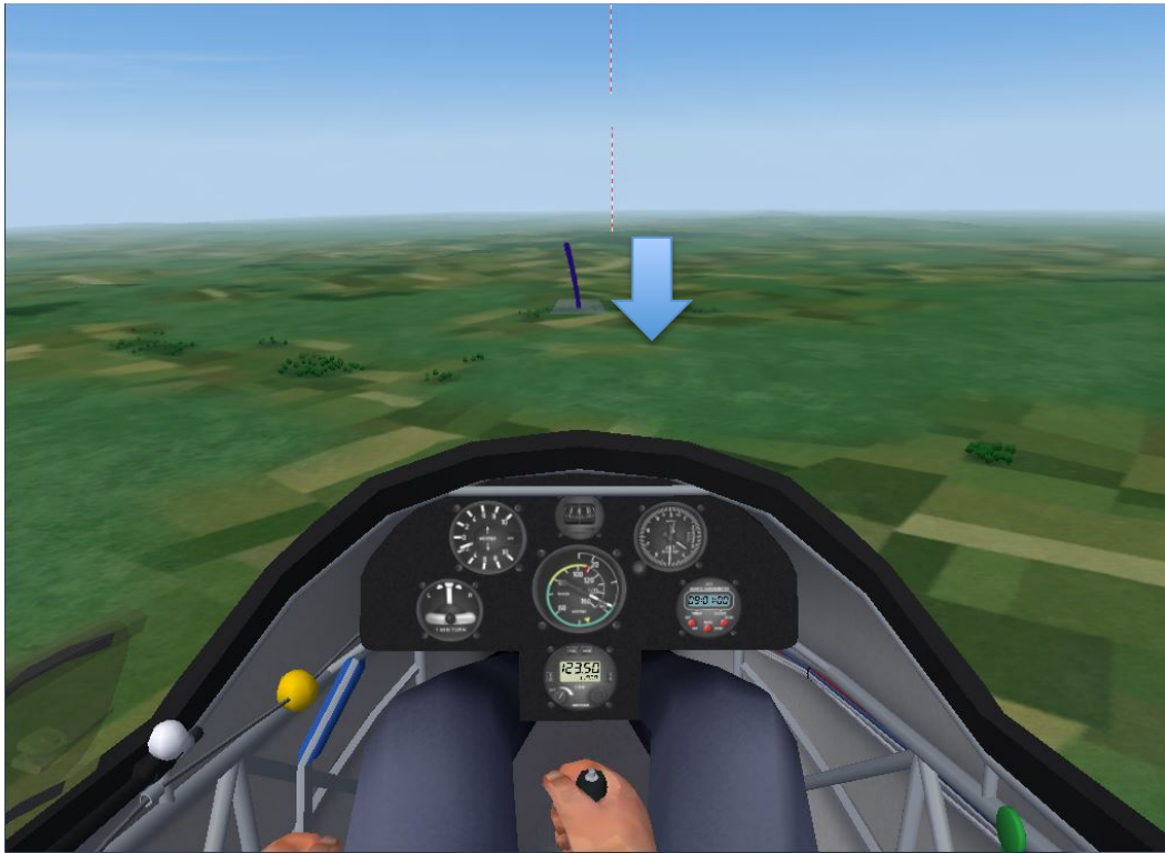
Initial pitch below the attitude required for 42 knots
