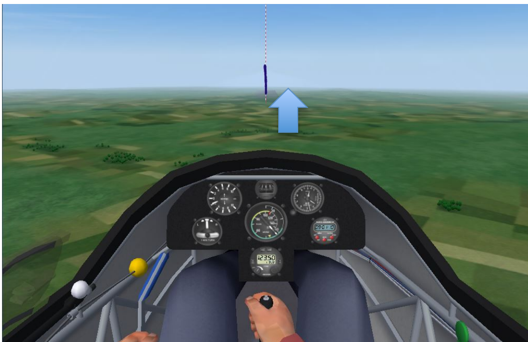
Secondary pitch to capture/hold the 42-knot attitude
